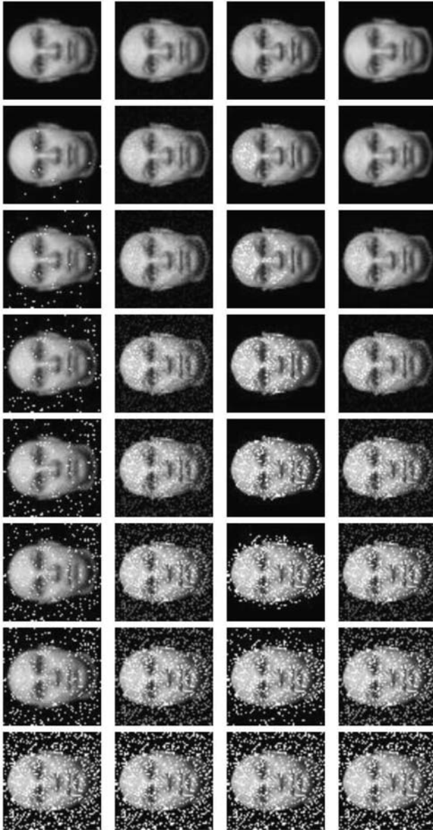
Fig. 5 “Complete corruption” scenario. The pixel-by-pixel denoised images, i.e., \mathbf{x} + \boldsymbol{\alpha} , using LAD-LASSO (first row), LS-LASSO (second row), LAD-Adaptive-LASSO (third row) and LS-Adaptive-LASSO (fourth row). Different images correspond to different values of s (from small to large)
